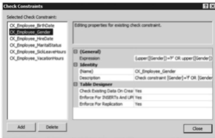
**Figure 1-5** A database constraint
